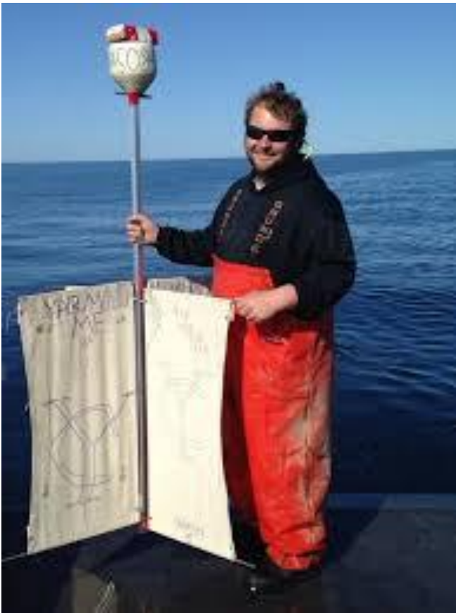
Figure 13. An Irina satellite-tracked surface drifter. The lower canvass drogued component is below the sea surface.
